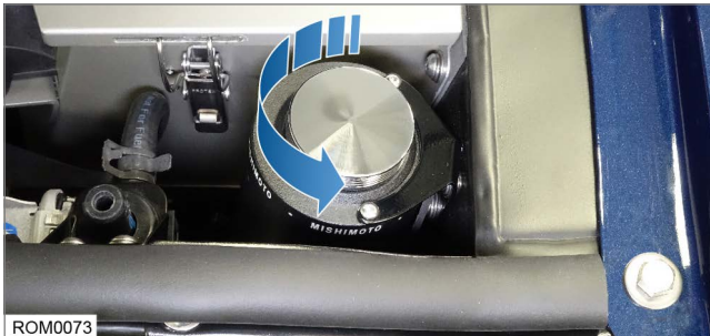
Unscrew expansion tank cap.
