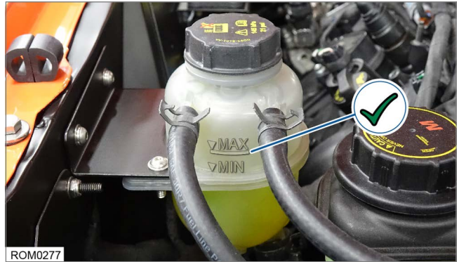
The coolant level in the expansion tank should be approximately half full when the engine is off and the system is cold. Reinstall cap when done checking/filling.
