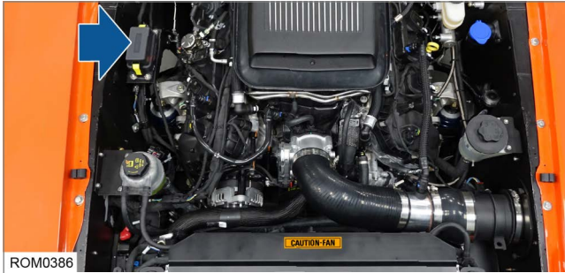
The engine compartment fuse center is located on the right apron.
